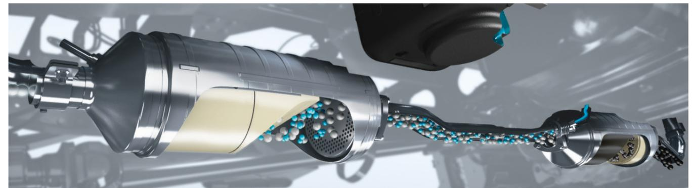
**The emissions control system.** All engine variants have a closed, maintenance-free diesel particulate filter which regenerates automatically – although you can do this manually if you need to. Exhaust gases are cleaned by a combination of oxidation catalytic converter and diesel particulate filter. Along with BlueTec® 6, the technology ensures all Canter models comply with the Euro VI standard.
