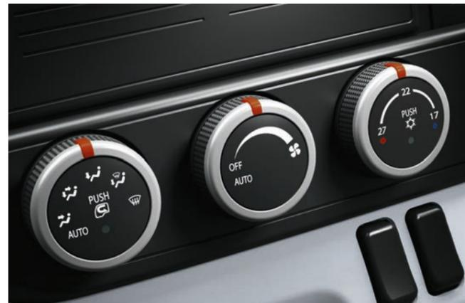
**The cab's climate control.** For ideal in-cab conditions we offer a choice of a manual air-conditioning system or optional automatic climate control. There's separately controlled ventilation for the crewcab.
