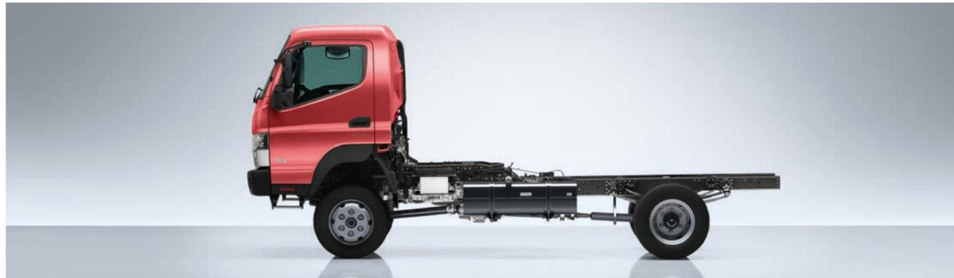
**Payload capacity.** The Canter 4x4 has a chassis load-bearing capacity of up to 3685 kg. With axle loads of up to six tonnes as well as an optional 24V interface and power take-offs ex-factory, a large choice of body options and solutions is available.
