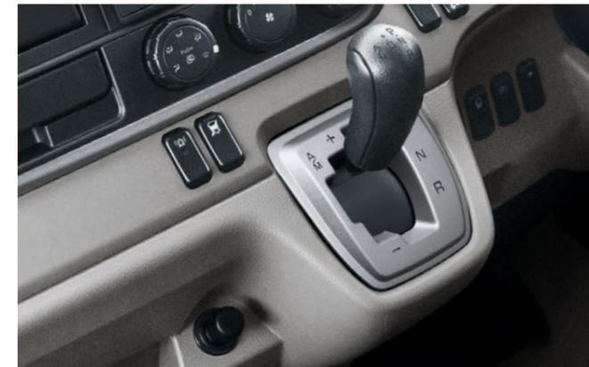
**Parking lock function and manual shift option.** DUONIC® offers a parking lock function to secure your Canter when it's parked. You also have the option of manually shifting up and down through all six gears.
