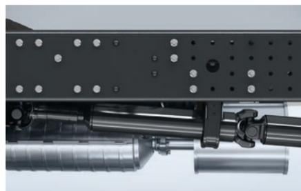
**The frame – robust and flexible.** A common hole pattern on the ladder-type frame for all models makes the Canter extremely versatile, making it easier to attach a wide range of bodies. The optional 24-volt interface and various power take-offs available ex-factory – for driving hydraulic pumps or compressor units – ensure the Canter is game for anything.
